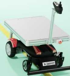
Line Trace Mode Retro-Reflective Line Tracking Navigation
